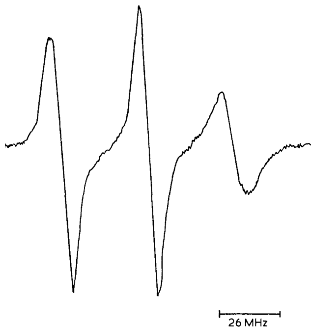
Figure 4 E.s.r. spectrum of labelled polymer from p -chlorostyrene copolymer after reaction with BuLi/TMEDA and MNP in benzene solution
